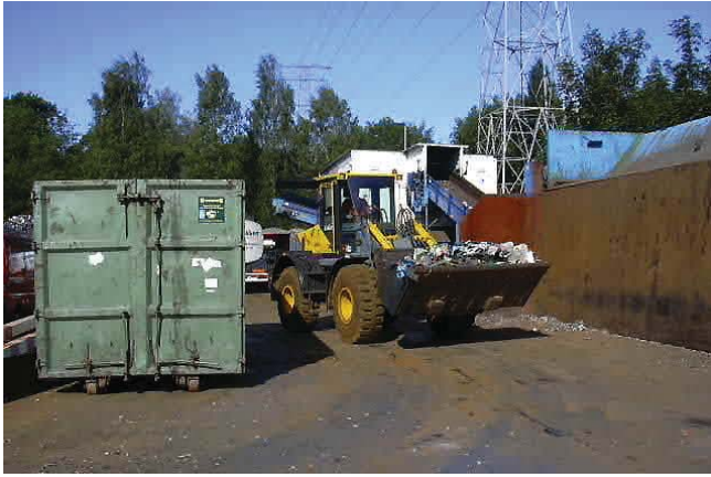
Exhibit 5.8 WEEE fed to 'opening' shredder
